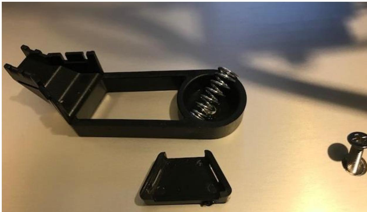
19. Install the supplied cable organizer and bed mount and use the slots on the mount to install new zip ties as shown below. Below is an Ender 3 but the steps are identical.
