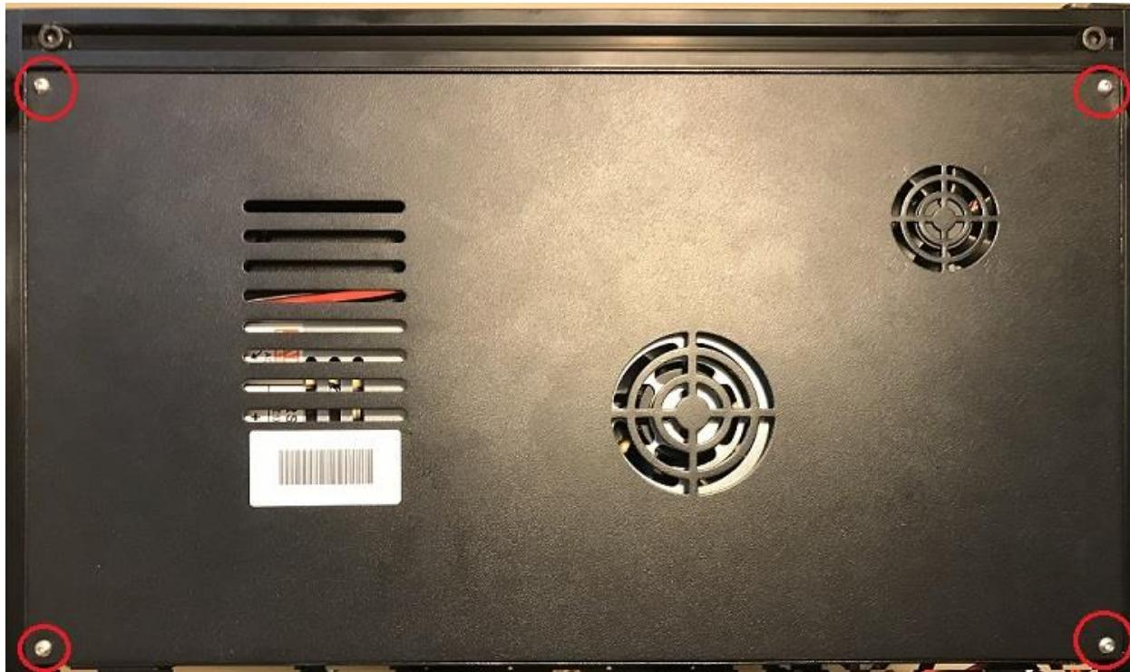
5. Move the case cover off to the side to expose the motherboard.
